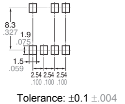
Recommended mounting pad (TOP VIEW)
