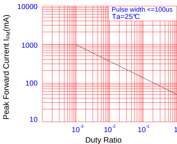
Fig.5 Peak Forward Current vs. Duty Ratio
